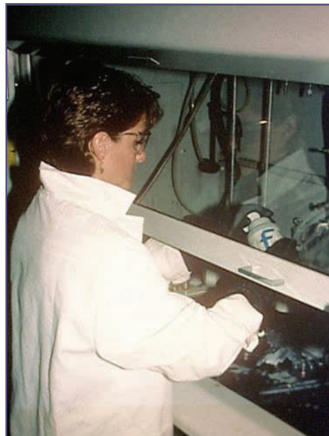
Proper use of a chemical fume hood equipped with a vertical sash.
